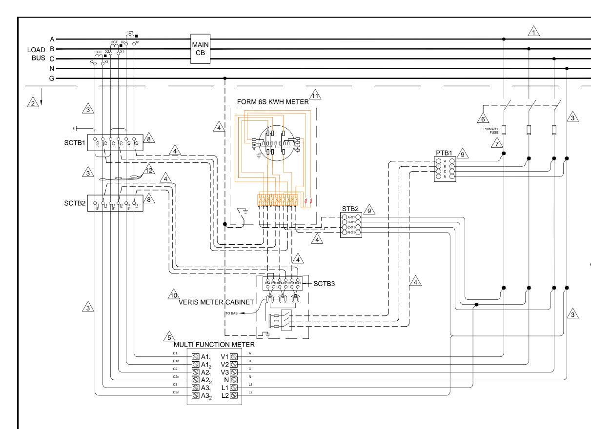
EQUIPMENT AND WIRING SHOWN WITH SOLID LINES SHALL BE PROVIDED BY SWITCHBOARD MANUFACTURER AND BE FACTORY WIRED.
